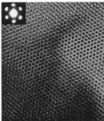
Figure 1. Transmission electron micrograph (inset: electron diffraction pattern) of FSM-16.
